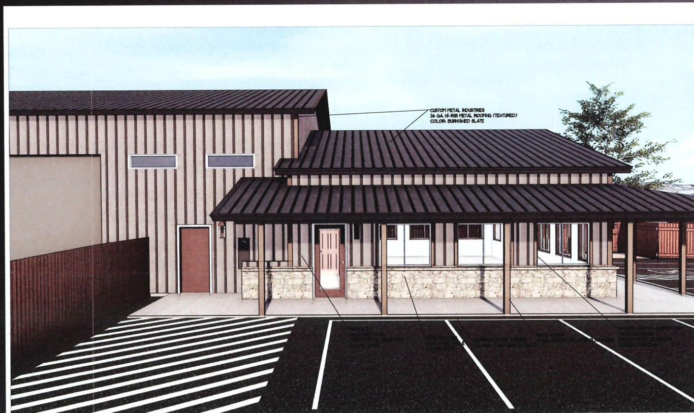
NORTH ELEVATION - METAL SIDING
