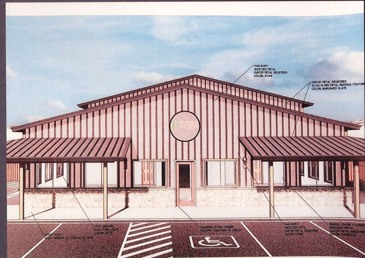
WEST ELEVATION - METAL SIDING
