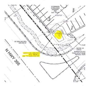
There is an existing storm drain along the front of the property which the sites overflow will be tied to. The storm drain leads to the Cottonwood Slew. The Town will not be responsible for maintaining the onsite storm water and will require a maintenance plan as per a condition of this report.
