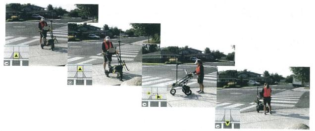
Next the wireless measuring wheel provides an **automated method to capture all the dimensions without having to manually enter any values**. Simply roll the surface, press capture and move on to the next dimension to be measured.
