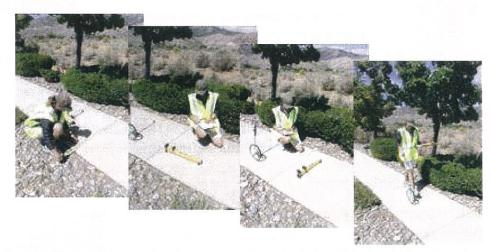
The pedestrian access route grade, cross-slope, and surface are measured continuously each time there is a change and maximum 25 ft. apart. Grades are recorded when they exceed the general grade established for the adjacent street or highway and they exceed 5%. The distance over which the grade occurs is also recorded. Cross slopes are recorded if they exceed 2% in either direction and the distance over which the cross-slope occurs is also recorded.
