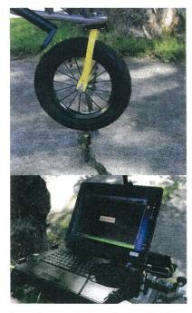
The PROWAP greatly increases the efficiency and accuracy of Trip Hazard detection and collection while reducing the **physical requirements** at the same time. The first advantage is that of detection. The PROWAP system is programmed with an algorithm that electronically monitors the sensor readings taken over time while traversing the Pedestrian Access Route PAR) and provides both audible and visible alerts when the cart impacts a vertical discontinuity greater than 0.25 in.
